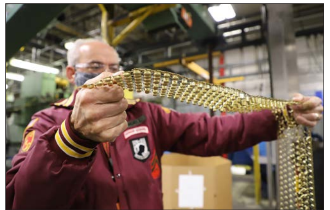
Federal retiree Dennis Angell, who has come back to help with hiring as production expands, holds up a piece of brass from which casings were made. The leftover brass gets sent to the supplier, melted down and used all over again.
