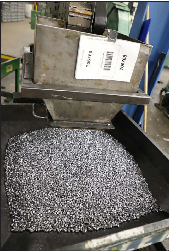
A machine cuts and forms the long cords into bullets, then drops them into a bin.
