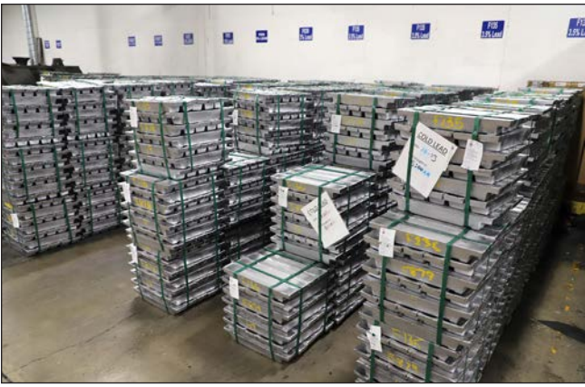
Antimonial-lead ingots are stored in three areas depending on how pliable they are. The more antimony in the alloy, the harder it is. The ones in this image are 1.5 percent, 3 percent or 3.5 percent antimony. The lead-antimony alloy is highly resistant to corrosion.
