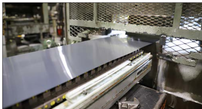
A machine cuts steel to be formed into primers for shotshells.
