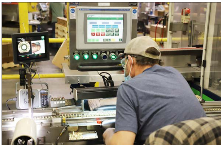
A worker and a computer both inspect each finished cartridge for the slightest blemishes. Federal has a photo of every round it makes.
