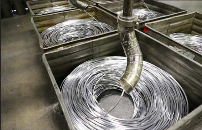
Even though it is technically an alloy, everyone still calls it lead. The lead is pulled into long cords and coiled for the next step.
