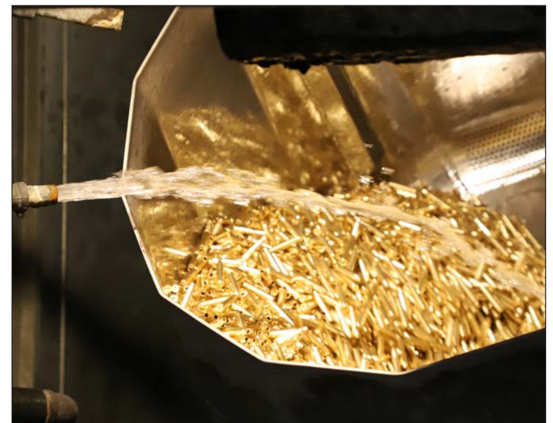
Everyone loves to see shiny brass when they tour the Federal plant in Anoka. Here, brass casings are washed in a tub.
